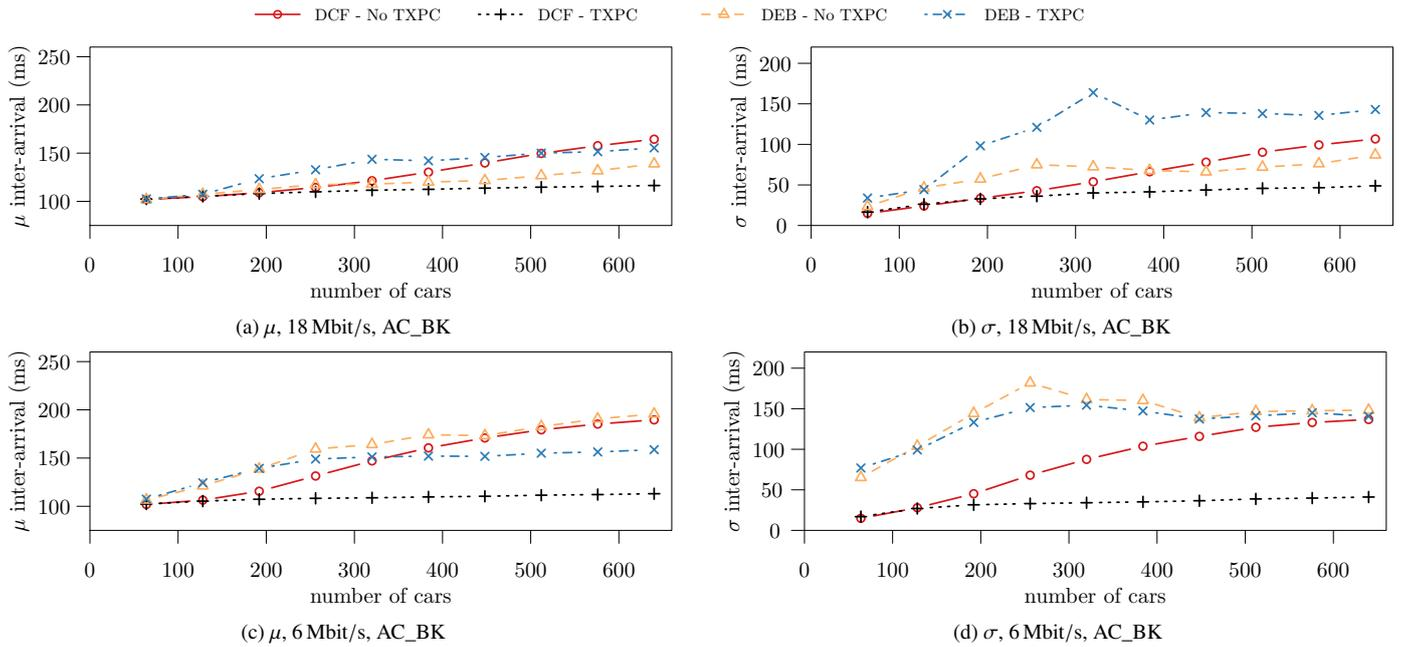
Figure 9: Weighted mean and standard deviation for front packets' inter-arrival time.
