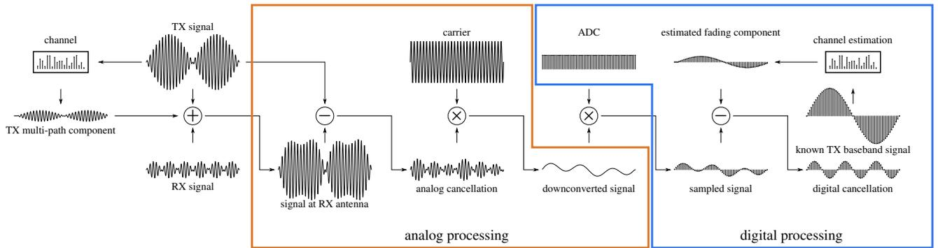
Figure 2: Simplified working principle of a full-duplex PHY.
