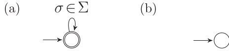
Fig. 2. Finite state automata acting as identity element and absorbing element for the automata cross-product operation. (a) Identity element. (b) Absorbing element.
