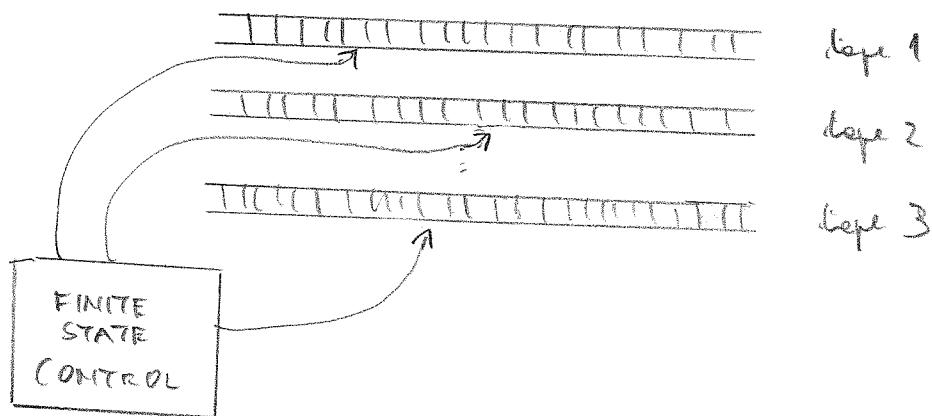
Initially: input  $w$  is on tape 1 with tape-head on the leftmost symbol. Other tapes are all blank.
