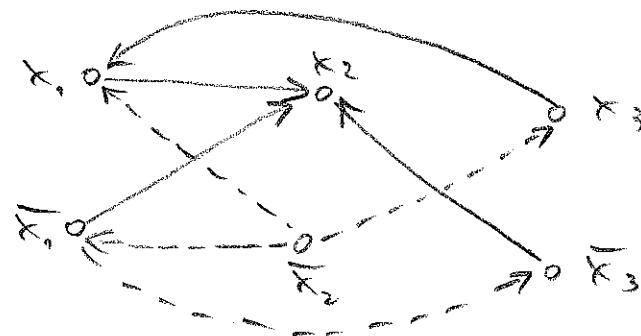
Then  $\Phi$  is unsatisfiable iff there is a variable  $x$  such that  $G(\Phi)$  contains two paths  $x \rightarrow \dots \rightarrow \bar{x}$
