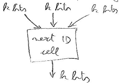
The next ID cell circuit depends only on the transition function  $S$  of  $M$ .  $\Rightarrow$  the size is constant.
