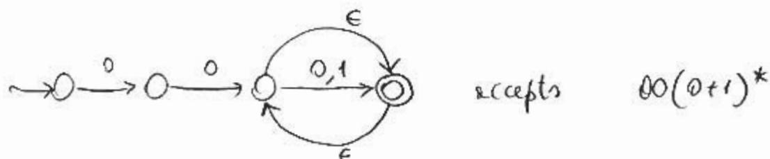
We can make the two rightmost states (with respect to the figure) collapse, thus eliminating the residual  $\epsilon$ -transitions:
