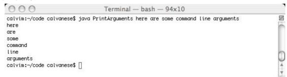
Note that the six strings "here", "are", "some", "command", "line", and "arguments" are the six arguments that are passed to the program when it is executed through the java command.
