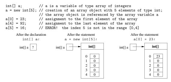
Note: It is very important to remember that, when an array contains N elements (N = 5 in the example), the indexes used to access the elements must necessarily be integers in the interval [0, N - 1]. Otherwise, a runtime error occurs when the program is executed. In the example, an error is signaled when the statement a[5]=16;
