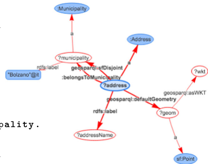
Fig. 7 The SPARQL query for “addresses registered in Bolzano but located outside” and its network representation
