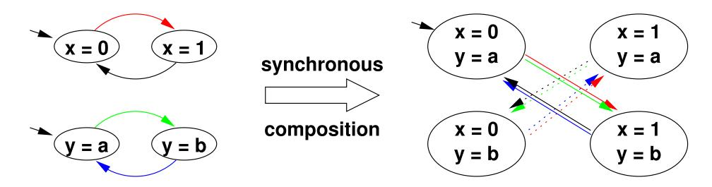
Typical example: sequential hardware circuits.
