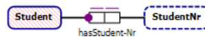
Fig. 2. ORM2 reference schema explained. Mandatory, graphically represented by a dot, and uniqueness constraints, represented by a continuous bar above the roles, are introduced.
