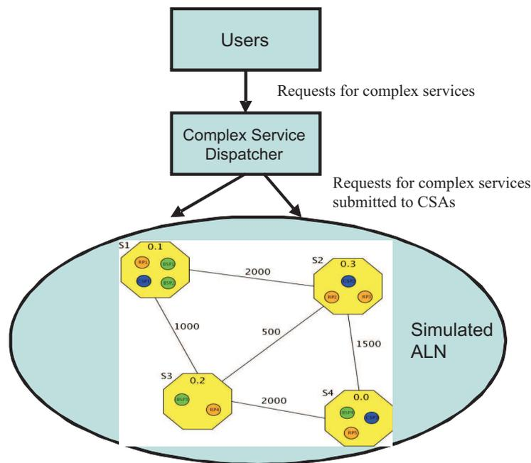
Figure 2. High level architecture of the CATNETS Grid simulator.
