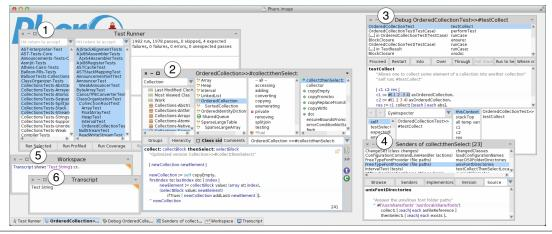
**Figure 1.** Standard Pharo Programming Environment with (1) Test Runner — for test driven development, (2) System Browser — a main tool for writing and reading source code, (3) Debugger, (4) SendersOf/ImplementorsOf/UsersOf — for navigating method and type references and declarations, (5) Workspace and (6) Transcript — for incremental and live programming.
