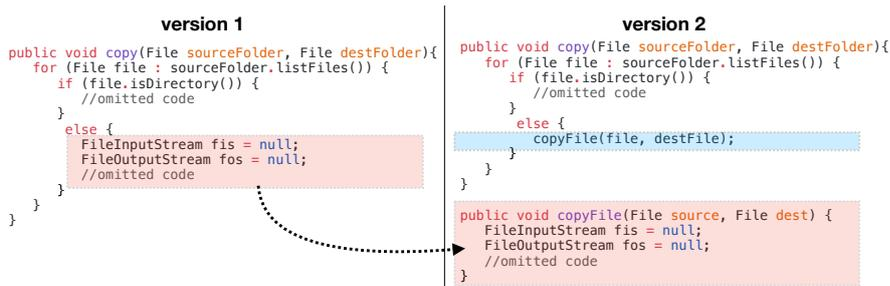
**Fig. 1** Example of the extract method refactoring.
