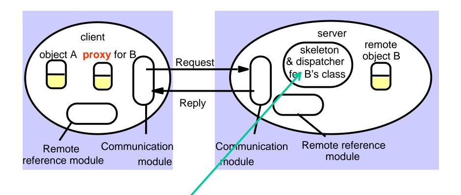
Dispatcher - gets request from communication module and invokes method in skeleton (using methodID in message).
