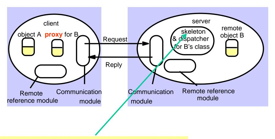
Skeleton - implements methods in remote interface. Unmarshals requests and marshals results. Invokes method in remote object.
