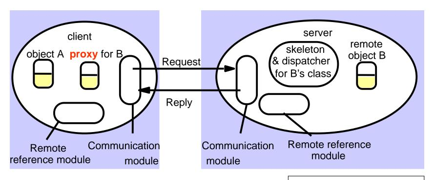
RMI software - between application level objects and communication and remote reference modules (according to JRMP v1.3)
