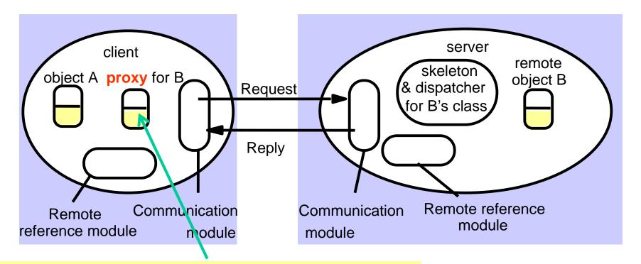
*Proxy* - makes RMI transparent to client. Class implements Remote interface. Marshals requests and unmarshals results. Forwards request.
