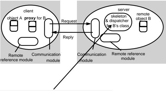
*Dispatcher* - gets request from communication module and invokes method in skeleton (using *methodID* in message).
