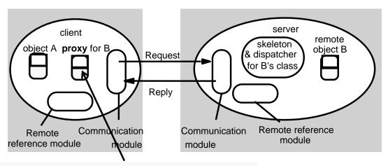
*Proxy* - makes RMI transparent to client. Class implements Remote interface. Marshals requests and unmarshals results. Forwards request.
