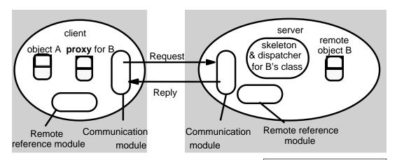
RMI software - between application level objects and communication and remote reference modules (according to JRMP v1.1)
