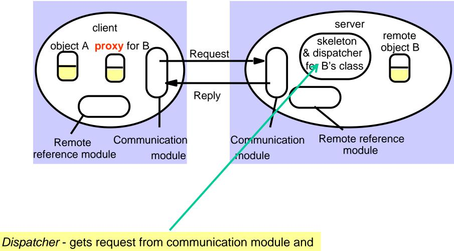
invokes method in skeleton (using *methodID* in message).
