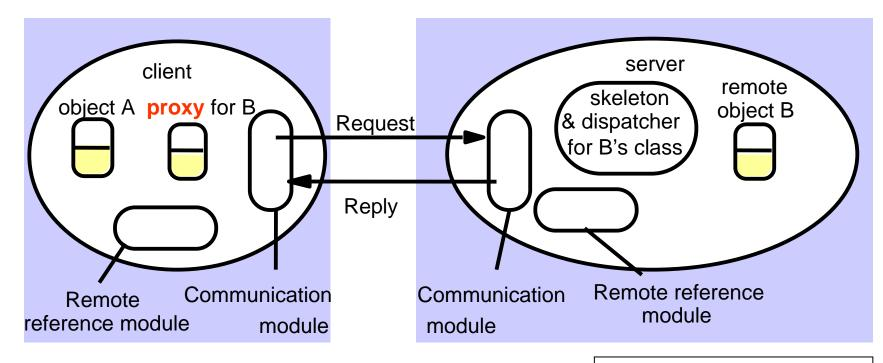
RMI software - between application level objects and communication and remote reference modules (according to JRMP v1.3)2
