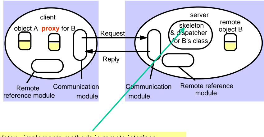
*Skeleton* - implements methods in remote interface. Unmarshals requests and marshals results. Invokes method in remote object.
