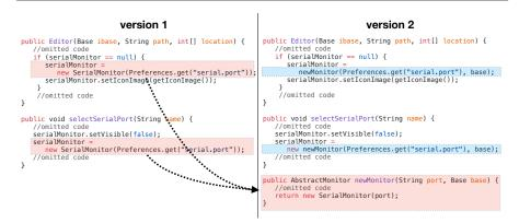
Fig. 3 Example of the extract method refactoring in which one method is extracted from two other methods.
