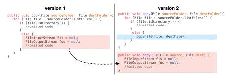
Fig. 1 Example of the extract method refactoring.
