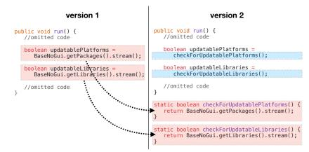
Fig. 2 Example of the extract method refactoring in which two methods are extracted from a single one.
